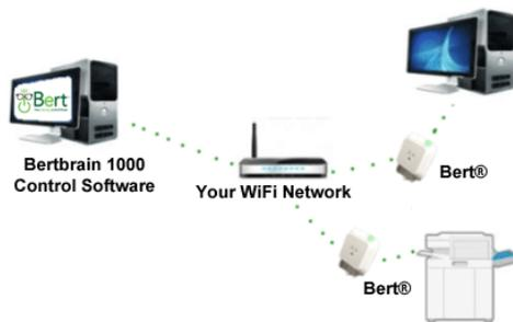
Each Bert® contains a microprocessor that can communicate with the Bertbrain 1000/M control software across your wireless network. Bert® can store 7-day on/off schedules with multiple on/off commands each day. This allows you to set schedules that mirror the actual operating hours of your facility and easily modify schedules throughout the year.
