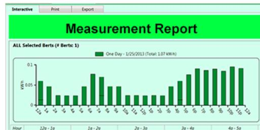
Facility managers can analyze the usage information to create optimal schedules to control plug based load using Bert®. The measurement tool has other benefits as well. Energy consumption and savings data can be used for budgeting or to verify performance contracts. During load shedding events managers can see the actual amount of power that is being saved during the event. Bert® measurement is a brilliant solution.
