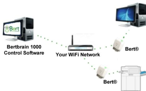
Each Bert® contains a microprocessor that can communicate with the Bertbrain 1000 control software across your wireless network. Bert® can store 7-day on/off schedules with multiple on/off commands each day. This allows you to set schedules that mirror the actual operating hours of your facility and easily modify schedules throughout the year.
